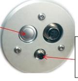
IP67 Rated M8 Connector for 12V nominal solar panel or provided external +24VDC charger.
